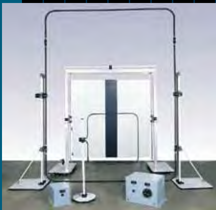
IEC 1000-4-8 Test Equipment
