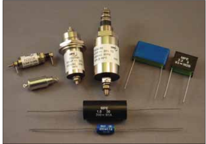
Figure 2. Typical feedthrough capacitors compared with two-terminal capacitors.
