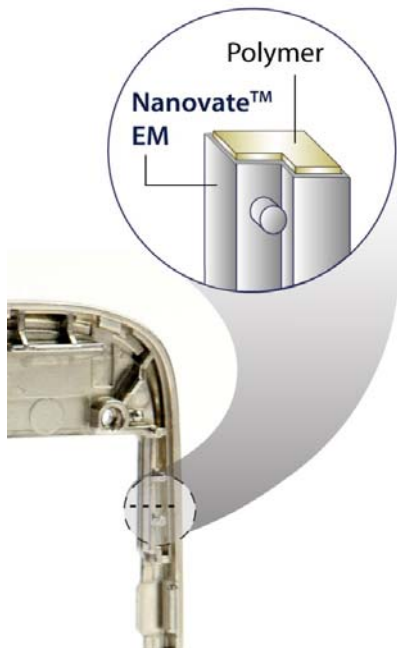
Figure 7 - Polymeric cell phone components coated with nanocrystalline Nanovate™ shielding. Source: Integran Technologies Inc.
