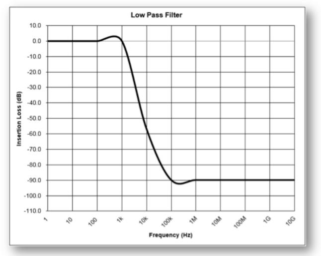
Generally AC Power systems run at either 50 Hz, 60 Hz or 400 Hz, so all Genisco Power Filters are Low Pass Filters. Our filters allow the lower frequency power signals to pass through the circuit, and block the unwanted higher frequency noise.
